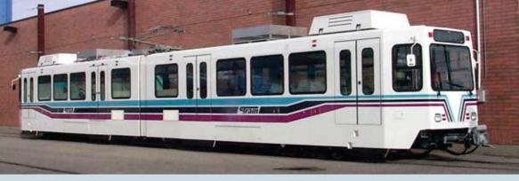
Bi-directional, six-axle, high-floor single articulated light rail vehicle constructed of low alloy high tensile (LAHT) steel, suitable for high platform operation.
