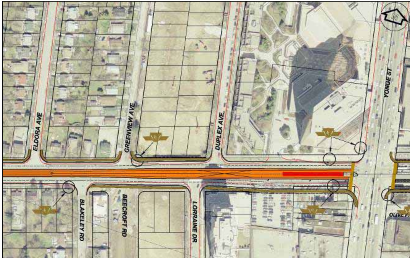
Exhibit 2-10: Option S1: Centre Station Platform on Surface
