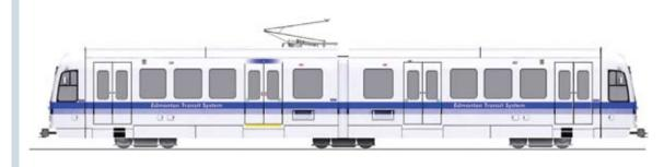
The vehicle is a bi-directional, six axle, single articulated, high floor vehicle, suitable for high platform operation. The carshell is constructed of low alloy high tensile (LAHT) steel. The vehicle sections consist of two body sections and an articulated section.
